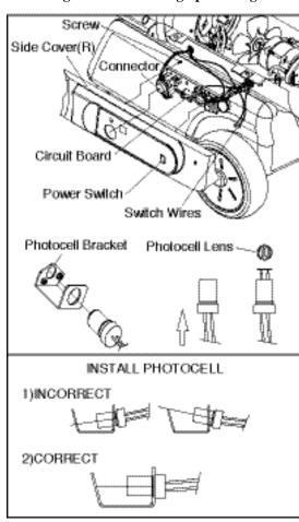
Figure 17. Replace & Cleaning Photocell
